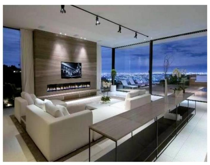
Lots of light in this California beauty 11ft wide, we added a high input to this design to allow plenty of flame due to the bright surroundings. This required additional venting to allow the unit to run cool in this warm climate.
